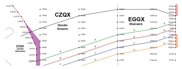
As can be seen, this routing remains laterally separated from track A (our most northerly NAT). Real life random routings should always remain separated from the NATs and would not be cleared if they cross. On VATSIM, this is left to the controller's discretion.
